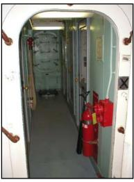
A major concern related to the simple task of walking down a passageway is the presence of bulkhead mounted equipment. Items mounted on a bulkhead, such as an electrical junction box or a fire hose box and fittings, present safety hazards. Further, it is advisable that passageways be kept free of any bulkhead-mounted objects if a passageway has any of the following characteristics (Zohar, 1978):
